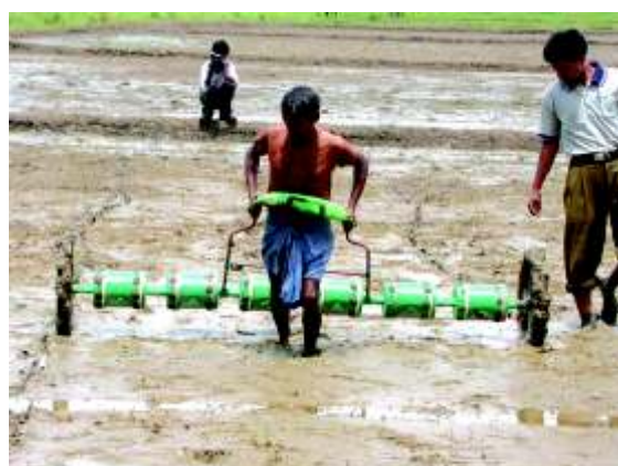
Sowing of pre-germinated rice seeds in puddled field through drum seeder
