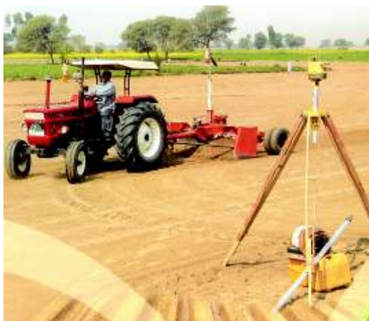
Laser aided land leveling in the field Source: Jat et al. (2006)
