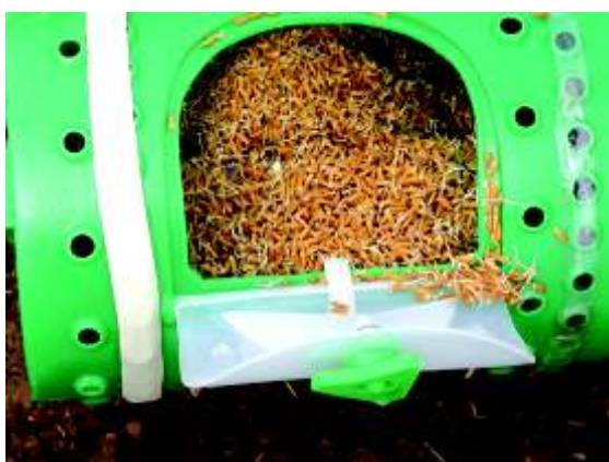
Box of Drum Seeder with Pre-germinated rice seeds
