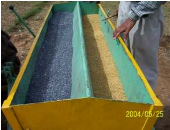
Separate boxes for seed and fertilizer in ZT drill machine
