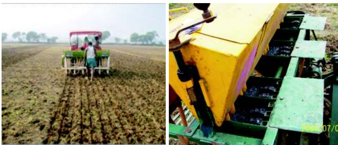
Zero tillage cum fertilizer drill machine and Zero Till Direct Seeded Rice (ZTDSR)
