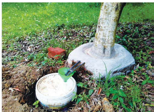
Fig. 15.2. Arrangement for measurement of stemflow
