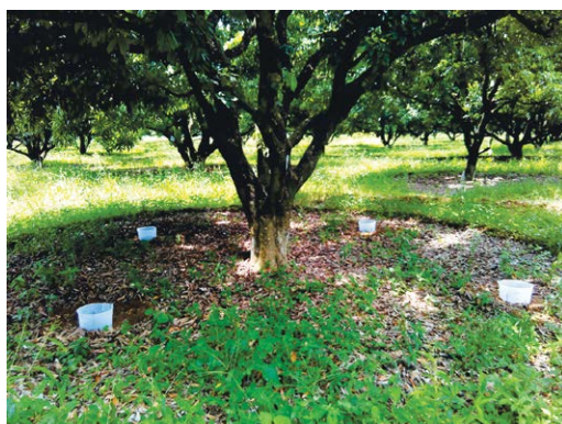
Fig. 15.3. Arrangement for measurement of throughfall
