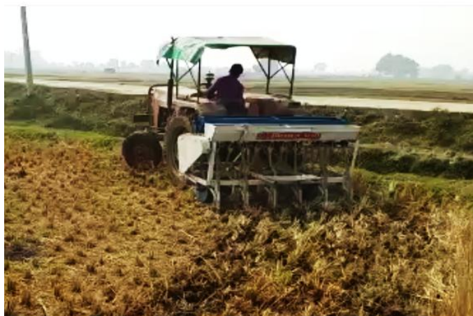
Fig. 3 Zero Seed cum fertilizer drill working in the field
