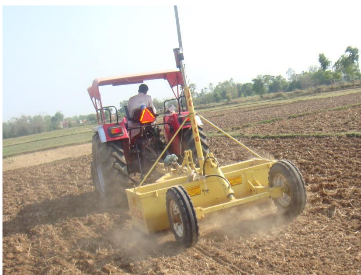
Fig.2 Leveling field by laser land leveler
