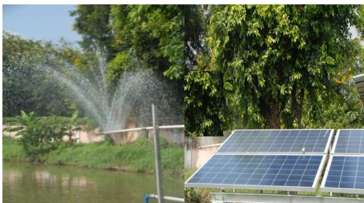
Fig 3. Spray type solar aerator for fishpond.
